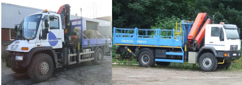
Typical steelwork delivery vehicles.
