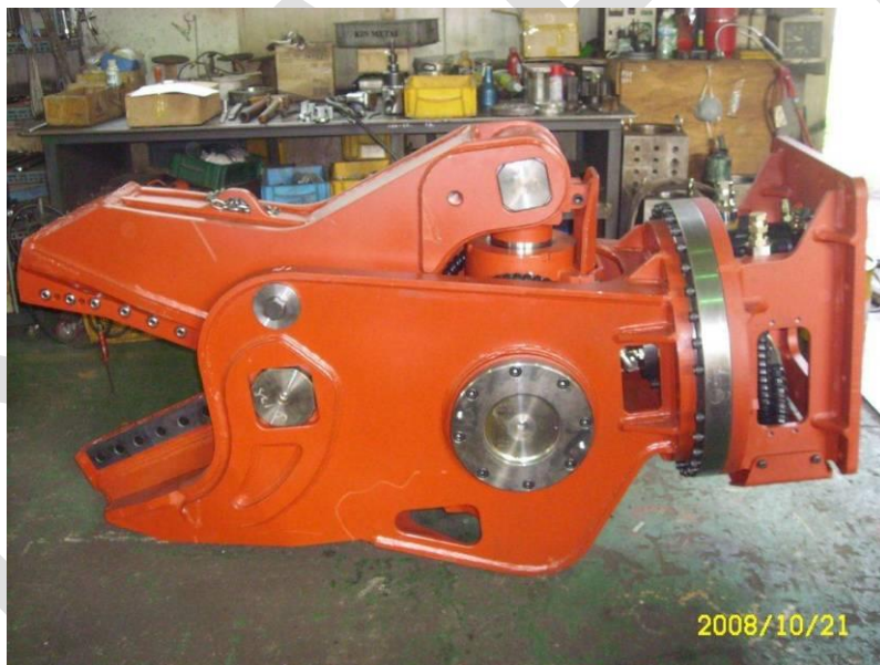
Large hydraulic steel cutting attachments
